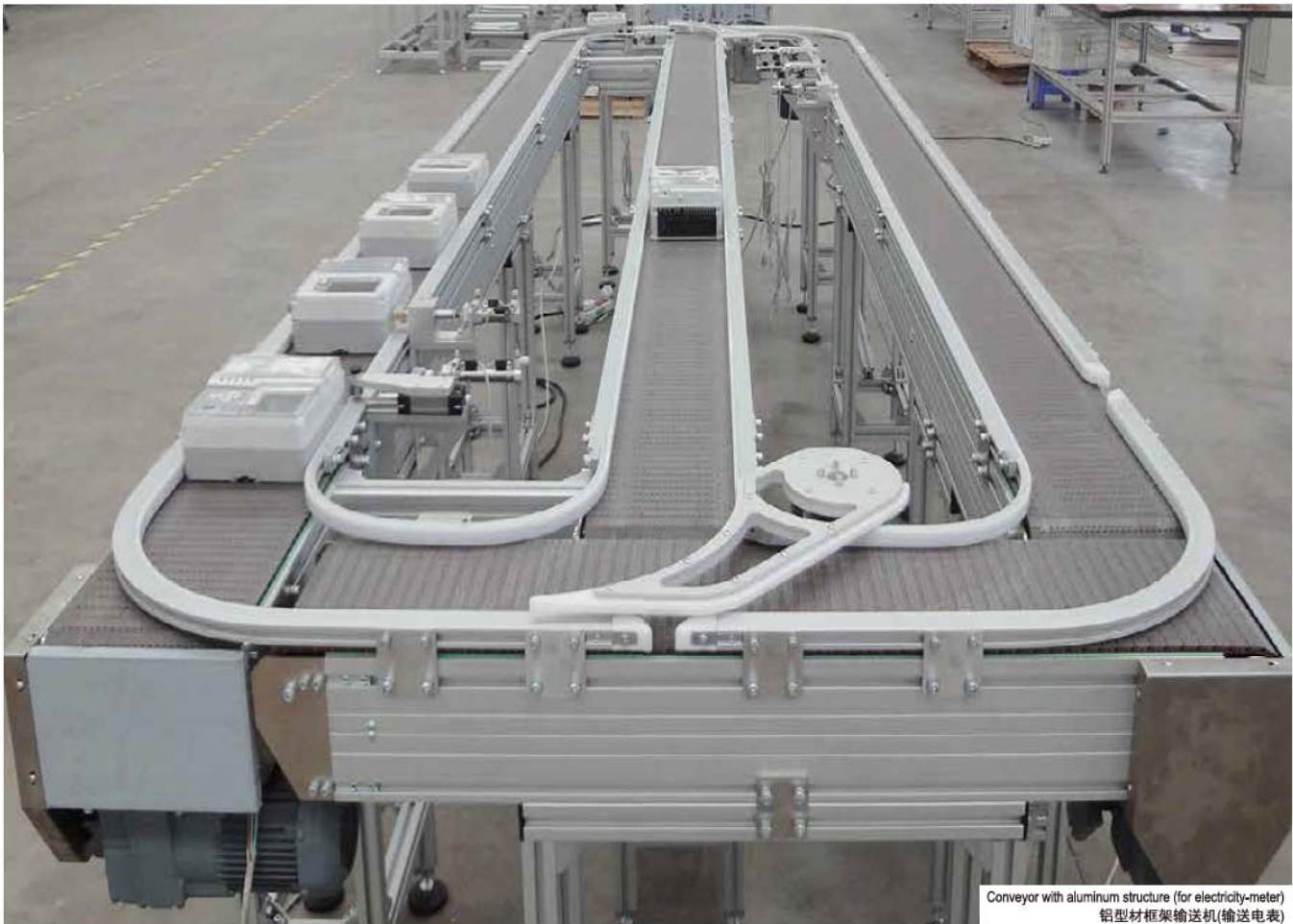
Conveyor with aluminum structure (for electricity-meter) 铝型材框架输送线(输送电表)
