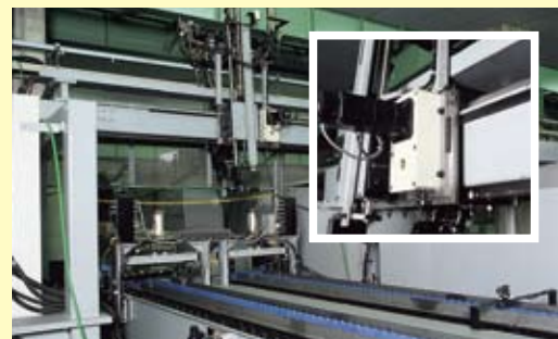
Automatic material handling equipment (CP racks & pinions)
